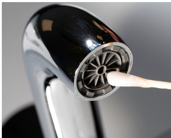
A sterile swab should be rubbed on the inside surface of the tap outlet or flow straightener
